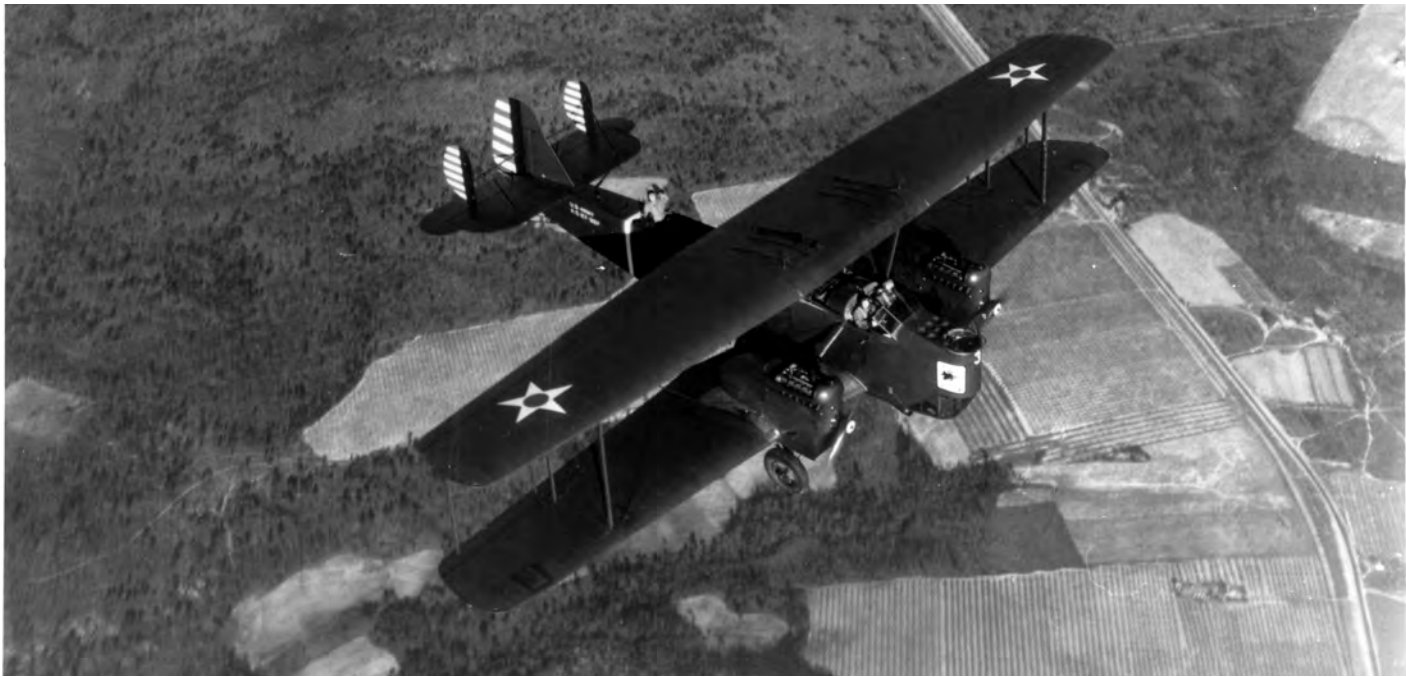
(Above) The first production version of the XLB-5 was the Keystone LB-5. The additional “stabilizing rudders” are readily apparent.
