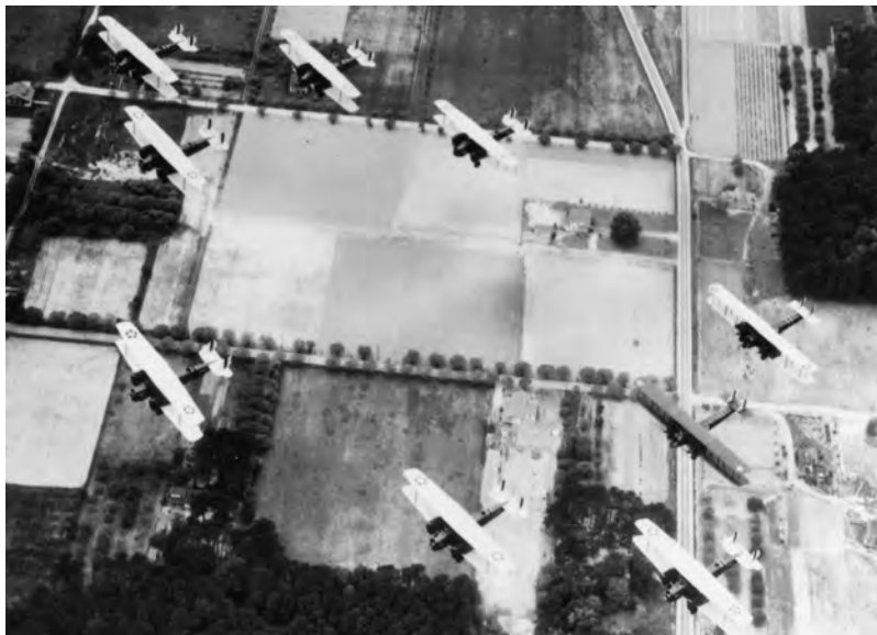
A year after the 1927 maneuvers, the 2d Bombardment Group's equipment had changed. This formation, on May 17, 1928, includes seven Keystone LB-5A bombers, identifiable by their tapered wings, and two Martin NBS-1s on the right.
