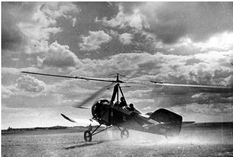
(Top) The SPL was equipped with an M-11 engine.
