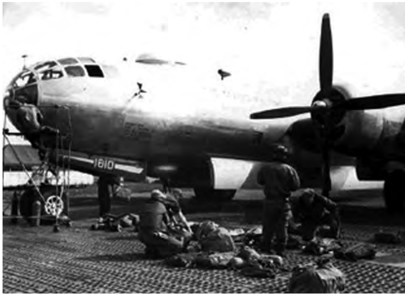
Preflight on RB-29 s/n 44-61810. "1810" was one of the "special photo" birds assigned to the 91st SRS' "C" Flight and its K-30 camera port is visible under the prop blade of #2 engine. (Bill Welch, The Cold War Museum, Vint Hill, Virginia)
