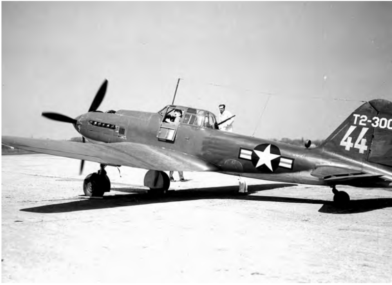
(Above) Two NKPAF Il-10s were captured intact at Kimpo AB in September 1950. One was used as the parts donor for this example to be evaluated by the USAF Air Technical Intelligence Center (later the Foreign Technology Division) at Wright-Patterson AFB, Ohio. It was flown 14.4 hours before a landing gear collapse terminated the USAF's first experience exploiting Soviet-built aircraft. (Photo courtesy of the Robert F. Dorr Collection.)
