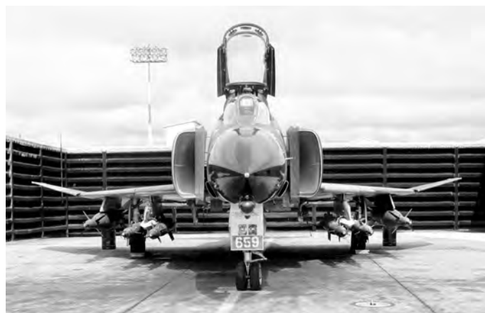
A heavily armed F-4D in its Ubon revetment. The aircraft, 67659 of the Satan's Angels (433rd TFS), is configured with a total of four Mk-82 and two Mk-84 Laser Guided Bombs.
