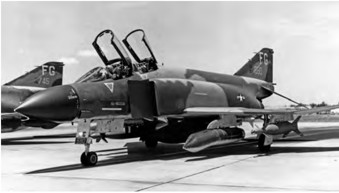
Goatee was scheduled as the third LGB flight on May 13 to strike the Dragon's Jaw. Goatee 01 were Lt Col Rick Hilton and Maj Bill Wideman of the 433rd TFS. The photo shows them in F-4D 67680/FG with KNIFE pod #4 and two Mk-84 LGBs on last chance.
