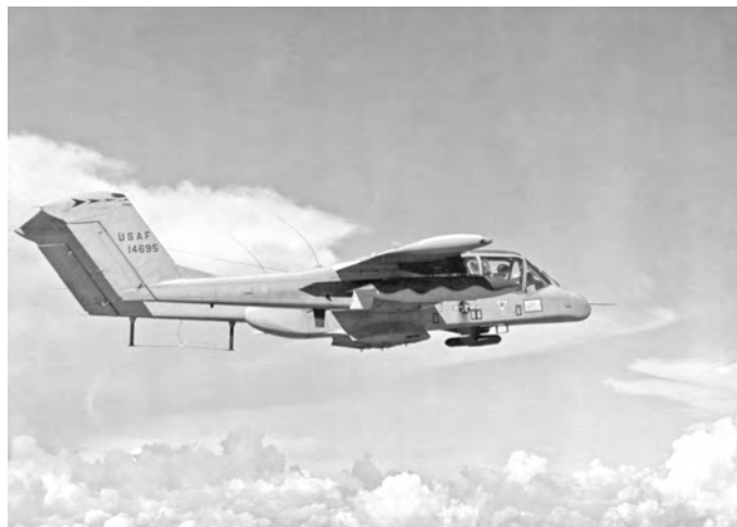
Combat Required Operational Capability (CROC) 25-70 was to modify fifteen straight OV-10A Broncos with among others ARN-92 LORAN-D with a modified computer and a laser ranger/designator. An OV-10 PAVE NAIL aircraft would be able to search, detect, track, range, and laser designate targets from a standoff position, at night. It would work in conjunction with LORAN/LGB-equipped F-4D aircraft of the 8th TFW. OV-10A 67-14695 of the 23rd Tactical Air Support Squadron, which had an Operating Location at Ubon, on this November 1971 photo carries a laser designator pod under its fuselage.
