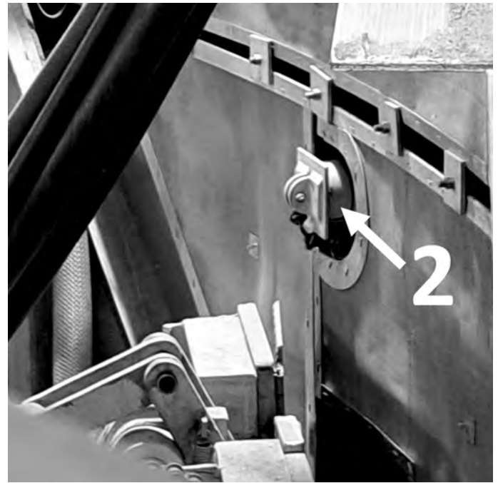
Figure 35: New Umbilical Release System. The solution to the lanyard failure was to replace the rigid D-ring attachment point on the launch dock wall with a flexible, J-shaped bar. The J-shape allowed it to flex slightly when the release lanyard pulled taut, permitting the mechanism to release. The umbilical pull problem did not reoccur. Courtesy of F.C. Radaz.
