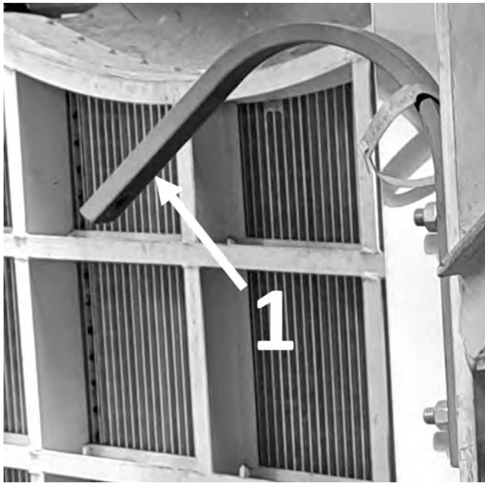
Figure 35: New Umbilical Release System. The solution to the lanyard failure was to replace the rigid D-ring attachment point on the launch dock wall with a flexible, J-shaped bar. The J-shape allowed it to flex slightly when the release lanyard pulled taut, permitting the mechanism to release. The umbilical pull problem did not reoccur. Courtesy of F.C. Radaz.
