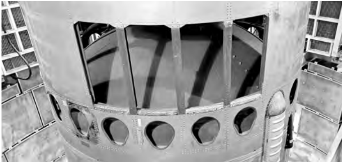
Figure 15: (Above) Titan II Stage II Exhaust Vents. The system of vents facilitated “fire-in-the-hole” staging by quickly venting the Stage II engine exhaust. Author’s Collection.
