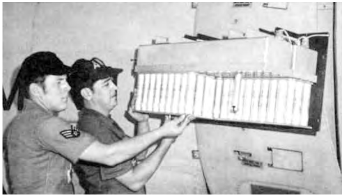
Cloud-seeding device being installed on the side of an unspecified USAF aircraft.
