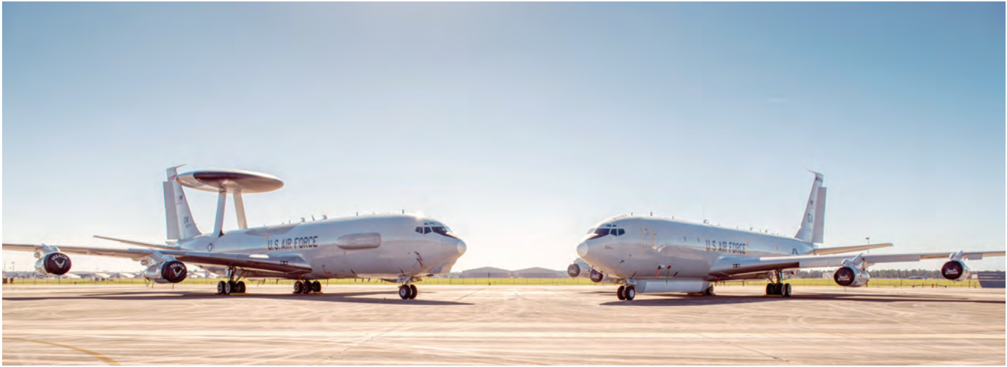
Boeing E-3 Sentry Airborne Warning and Control Systems (AWACS) and Northrop Grumman E-8 Joint Surveillance Target Attack Radar System (JS-TARS) together on the tarmac.
