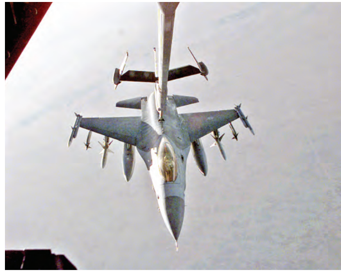
When the 561st FS Det at Dhahran redeployed to Nellis in early October 1994, it was replaced for the first time by a F-16CJ Wild Weasel Detachment of personnel and six F-16CJs of the 79th FS of Shaw's 20th Fighter Wing. The photo shows an F-16CJ, configured with AIM-9s, AIM-120s and AGM-88s, being refueled by a KC-10A Extender near the Iraqi border. [USAF, A1C Greg Davis]
