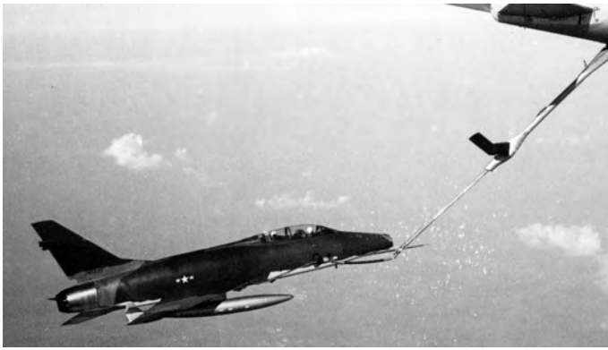
The F-100F's air to air refueling system was different than that used by other USAF aircraft flying into North Vietnam, complicating aerial tanker scheduling. (U.SAF photo.)
