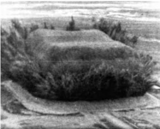
Figure 11. HEST II shortly after detonation. The overburden could be lifted as high as 180 feet depending on the amount of Primacord used. One complication was the need to remove all the overburden from the surface to investigate the damage, if any, to the test structures. (Courtesy of Boeing Company.)
