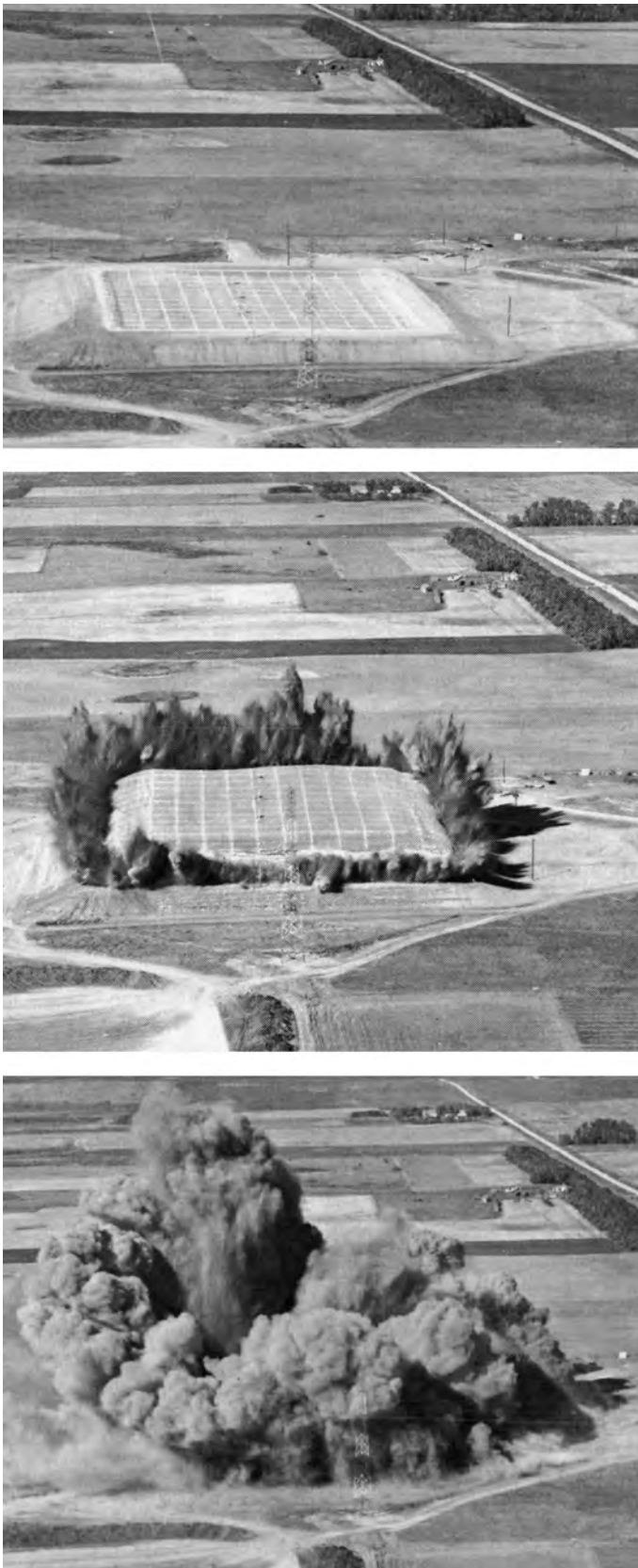
Figure 13. Upper: HEST III one second before detonation; Middle: one second after detonation; Lower: 15 seconds after detonation. (Courtesy of Boeing Company.)
