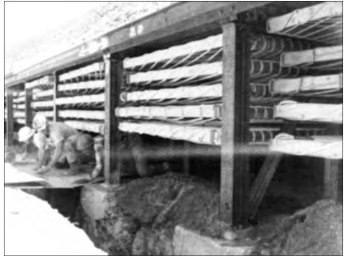
Figure 10. HEST II. Detail showing the layers of Primacord laced on 2x4 frames. (Courtesy of Boeing Company.)
