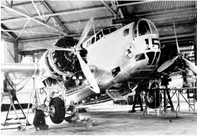
The Douglas B-18 was critical to the modernization of the Canal Zone's striking force. This 25th Bombardment Squadron B-18 is seen up on jacks in a hangar conducting landing gear maintenance. (AFHRA via George Cully.)
