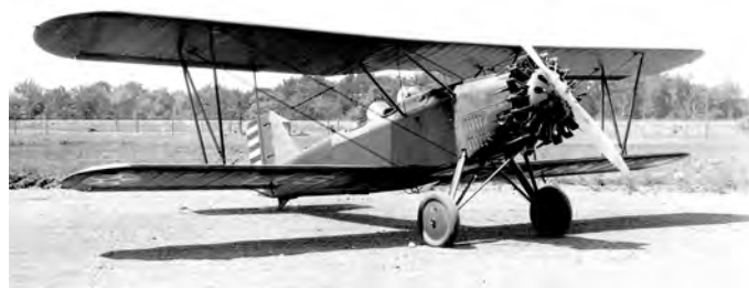
The Thomas-Morse O-19C replaced the Douglas O-2H in the observation role in Panama. Though the 7th Observation did not operate the O-19B shown in this photograph, the O-19C differed from the similar O-19B in having a tail wheel and cowling around the engine. (Photo courtesy of George Cully.)
