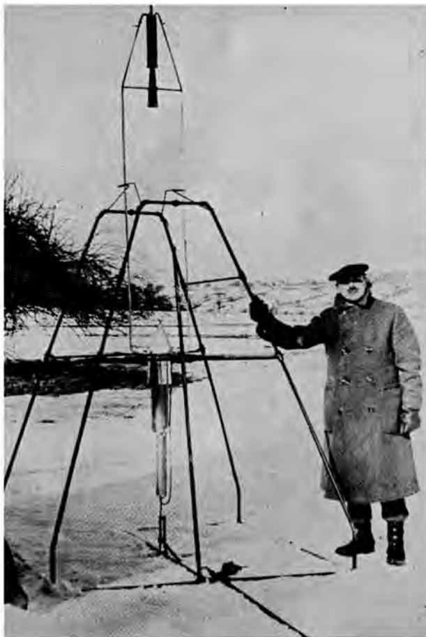
Dr. Robert H. Goddard standing beside the world's first liquid fuel rocket. This liquid oxygen-gasoline rocket was successfully fired on March 16, 1926, at Auburn, Massachusetts, what is now called the "Kitty Hawk of Rocketry."
