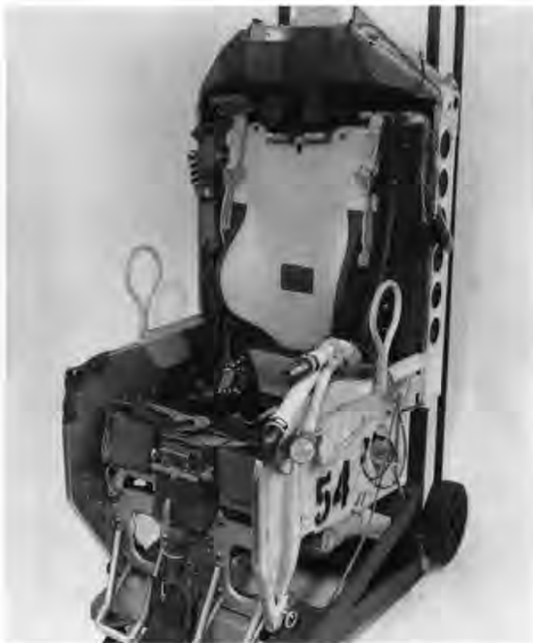
A 3/4 front view of the seat with arm guards deployed. Wheels are from a ground handling cart. A temporary recovery chute rests below the seat. (Photo courtesy of Gordon Cress).
