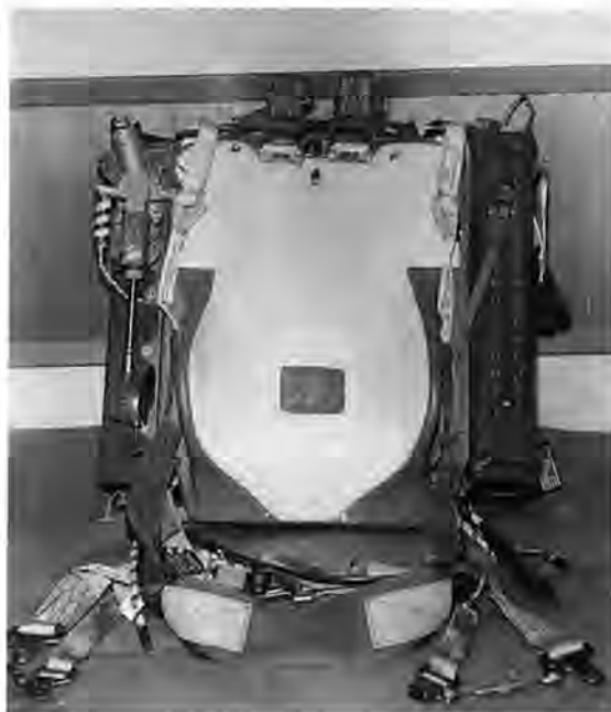
A front view of the backboard. Parachute drogue gun is on right side of seat with the barrel canted outboard and ballute pack is on the opposite side. (Photo courtesy of Gordon Cress).
