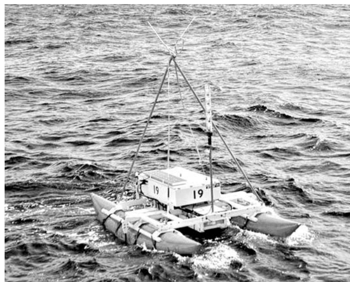
Figure 20. Livermore Independent Diagnostic Scoring System (LIDSS) instrument raft. (Courtesy Lawrence Livermore National Laboratory)
