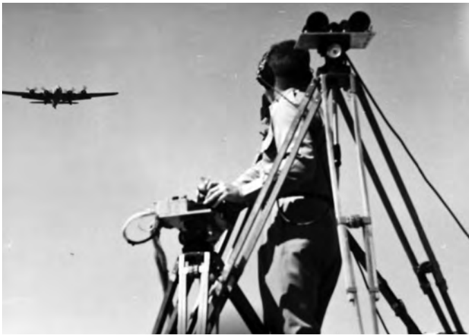
A QB-17 executing a remote landing. The rudder controller in the foreground guides the plane over the middle of the runway. The binoculars are needed to watch the drone as it is braked to a full stop further down the runway.
