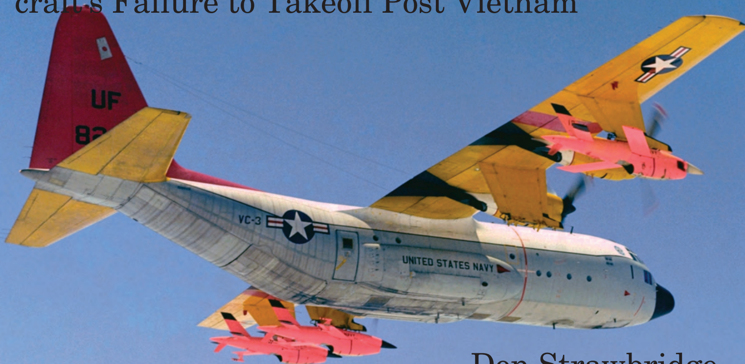
A U.S. Navy Lockheed DC-130A Hercules (BuNo 158228) from Composite Squadron VC-3 in flight in 1976, carrying subsonic Teledyne Ryan BQM-34S Firebee drones.
