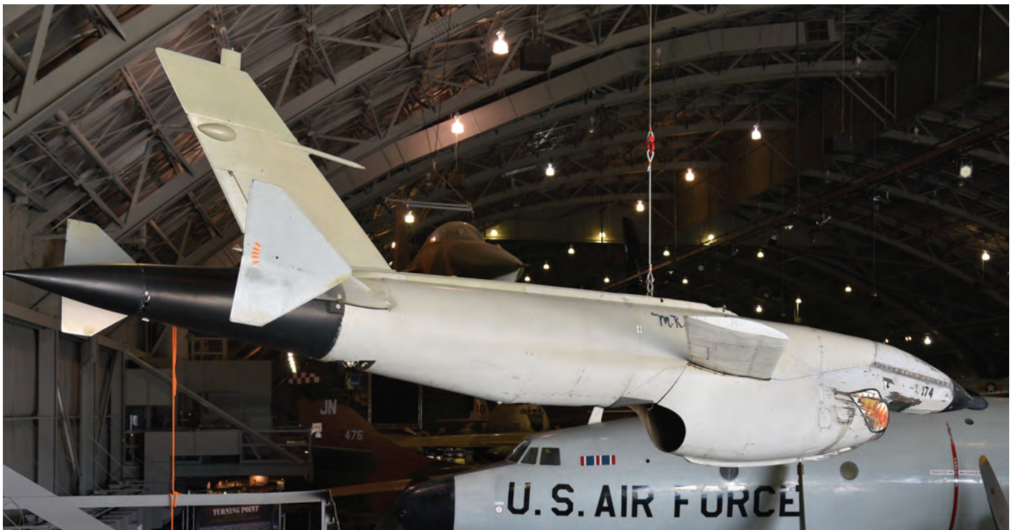
An AQM-34L hangs at the National Museum of the U.S. Air Force. The AQM-34L remotely piloted aircraft flew low-level photo-reconnaissance missions over North Vietnam. The AQM-34 series was developed from the unmanned BQM-34A target aircraft. The AQM-34L on display flew more than 30 missions over North Vietnam. This AQM-34L's nickname, M.R. Ling, was a pun on the last name of Lt. Col. Edwin Emerling, who was involved with its early combat missions. (NMUSAF/LaRock)
