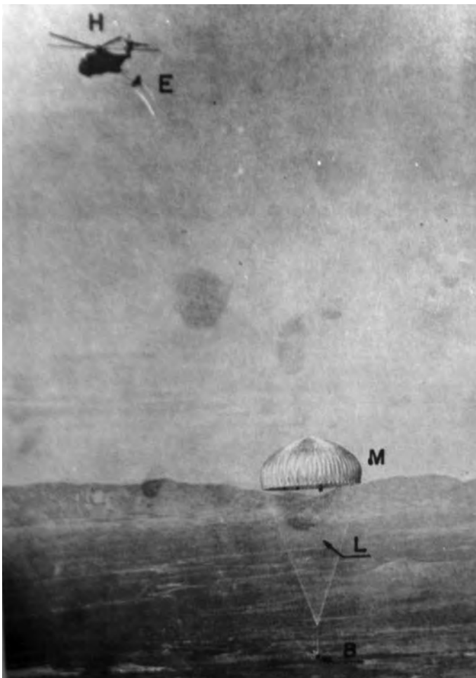
The Helicopter's Retrieval Hooks have Caught the Parachute Executing the MARS Process.
