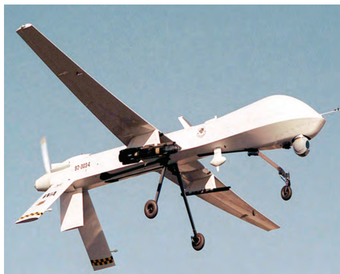
An MQ-1 Predator armed with an AGM-114 Hellfire missile flies a training mission. The MQ-1’s primary mission is interdiction and conducting armed reconnaissance against critical, perishable targets.
