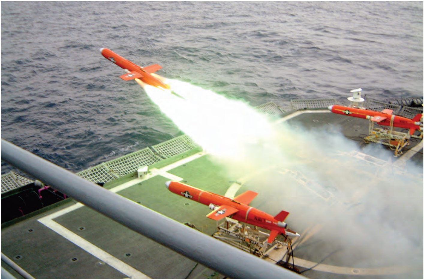
A BQM-74 Chukar target drone launched from the ship's flight deck and acted as a "hostile" anti-ship missile during a training exercise. ( United States Navy photo by Ensign Lyn Niemeyer. )
