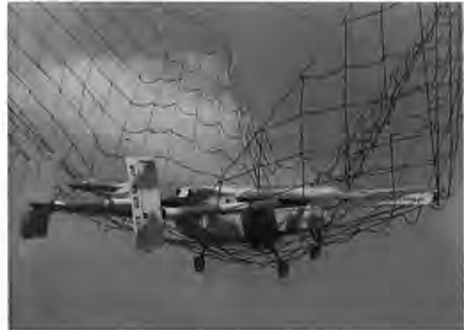
The Israeli Scout aircraft in flight. Note the underbody blister housing the television camera. The UAVs used in 1982 resembled this late model, but lacked the antenna for updated command and control data link. The SCOUTs that overflew the Beka'a Valley used a very simple data link, subsequently changed to avoid jamming and attempts to take over the aircraft by enemy units. Scout is retrieved in a net. (IAI photos)
